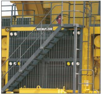
Komatsu's 960E-2 offers stairway access with entry from either the right or left side of the truck depending on the customer's preference.
