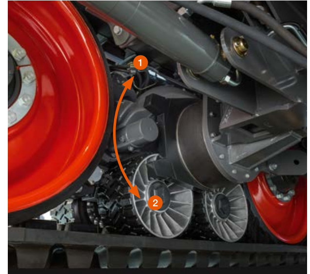
Robust pendulum stop 1 Oscillation range upwards 10° 2 Oscillation range downwards 13°
