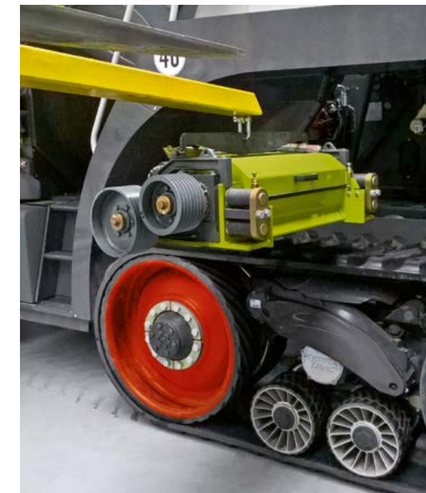
Straightforward removal of the corncracker above the crawler track unit
