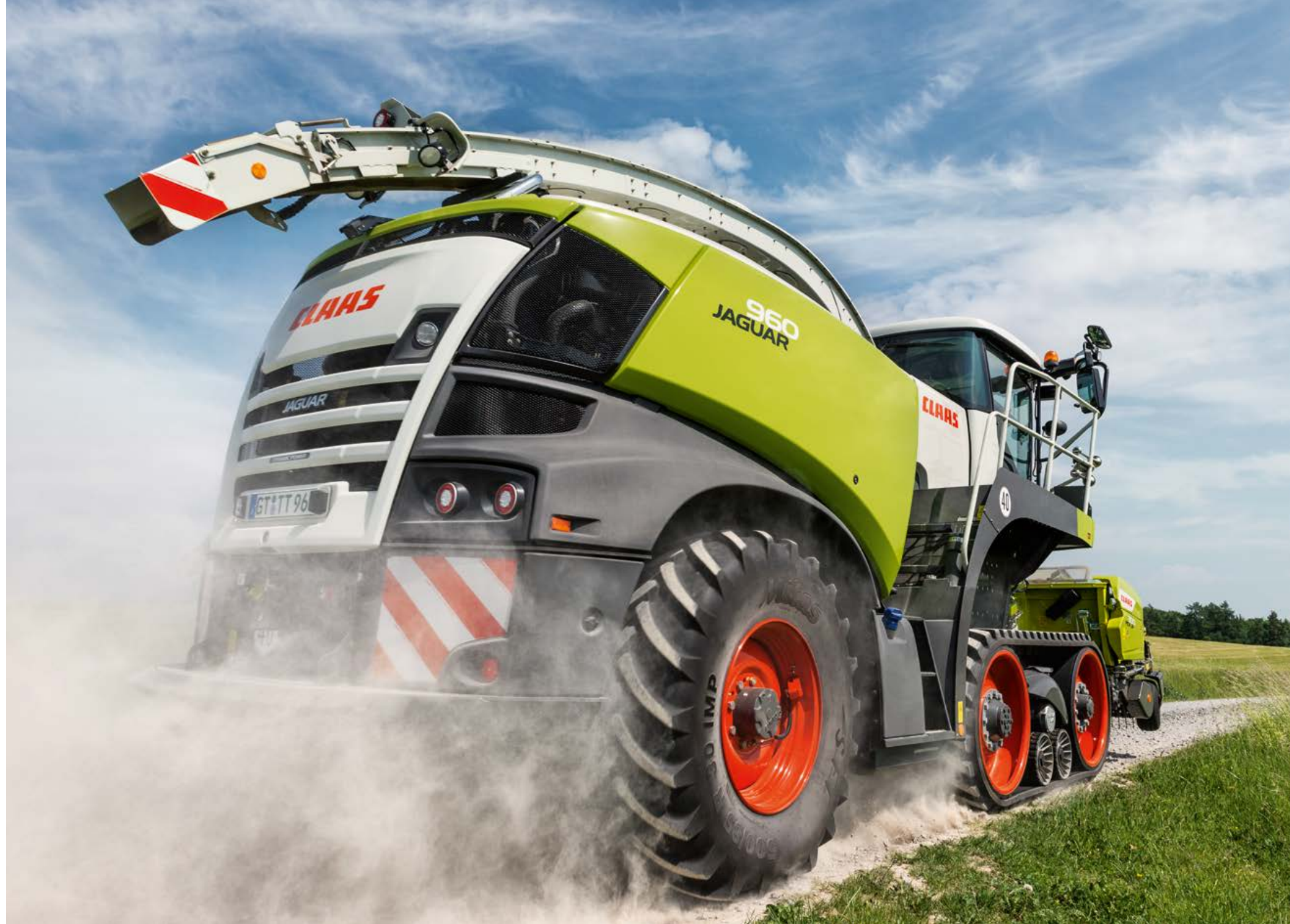
TERRA TRAC tracks are available in three widths for the JAGUAR
