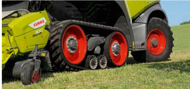
Raised crawler track at headland
