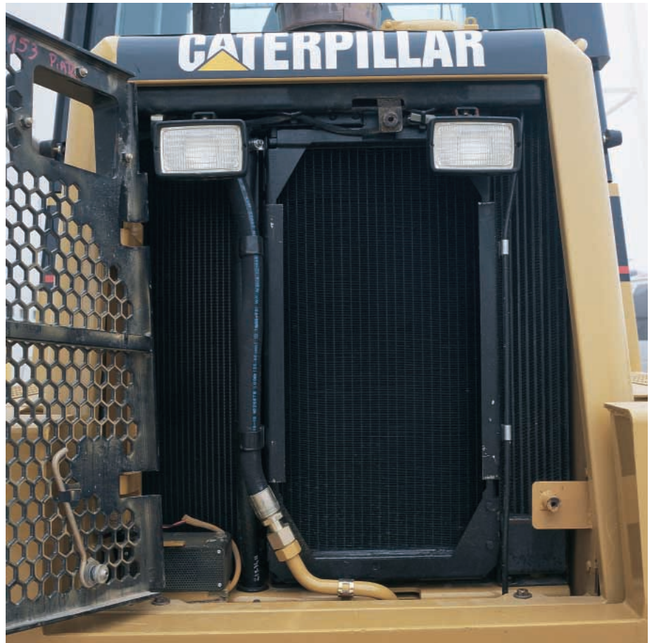
L/R: hydraulic oil cooler, engine radiator, air-to-air aftercooler
