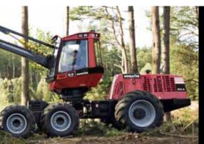
Stabilizer coupling and cab and boom leveling for optimum reach and stability
