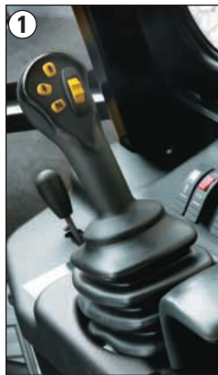
1 Pilot operated joystick with Forward/Neutral/Reverse switch and proportional auxiliary hydraulic control mounted on the joystick.
