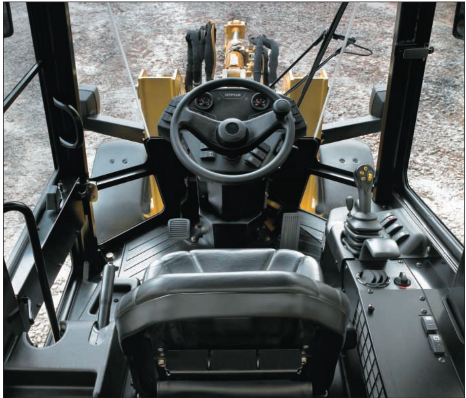
1 Pilot operated joystick with Forward/Neutral/Reverse switch and proportional auxiliary hydraulic control mounted on the joystick.
