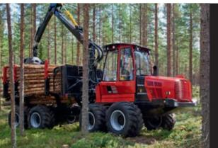
The new HST transmission with powerful traction of 193 kN gives increased performance through the unique interaction with the control system and the engine.
