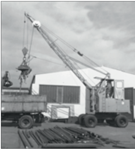
1962: rope-driven S833 with elevated operator cab
