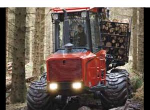
Superb mobility thanks to a steep nose angle, high ground clearance, low center of gravity, and low load height.
