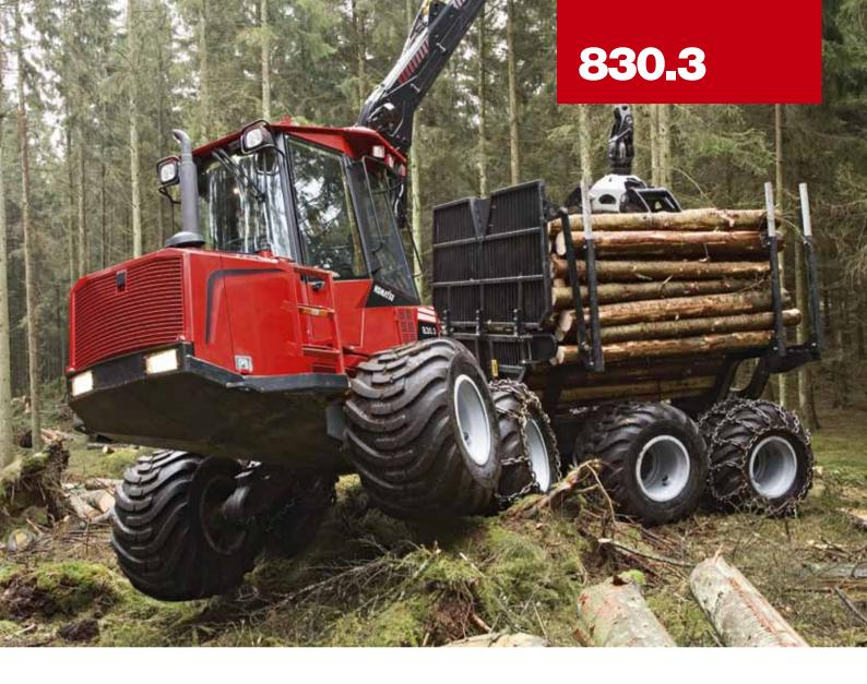
delivers ten percent more torque providing a full 600 Nm (440 lb-ft). This also applies to the already fast and nimble loader, with the lifting force increased from 67 to 74 kNm (49,400 to 54,600 lb-ft).
