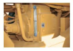
**Transmission Oil Fill Tube.** Is located beneath the platform area and the transmission oil dipstick has a sight gauge next to the fill tube for easy maintenance.
