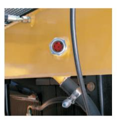
**Daily Maintenance.** Lockable ground level service doors give quick access to engine oil fill and dipstick, coolant sight gauge (above), rear frame grease fittings, relay panel and electrical breakers.
