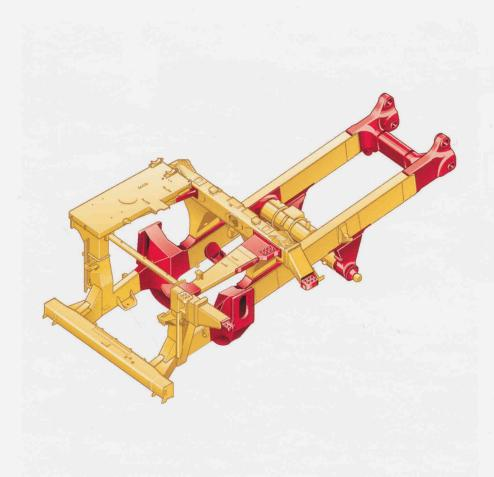
**Box-Section Design.** The 785C frame uses a box-section design, incorporating two forgings and 24 castings in high stress areas with deep penetrating and continuous wrap-around welds to resist damage from twisting loads without adding extra weight.
