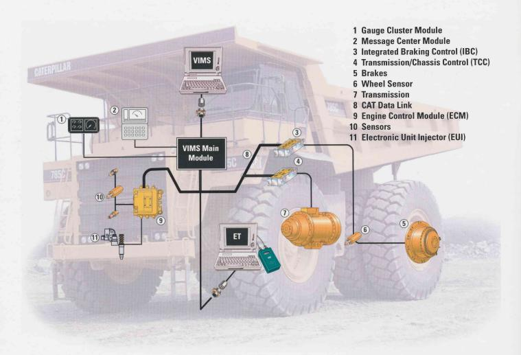
**Cat Data Link.** Electronically integrates machine computer systems to optimize overall power train performance, increase reliability and component life, and reduce operating costs.
