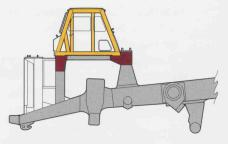
**Rollover Protective Structure (ROPS).** Integral to the cab and frame, ROPS is resiliently mounted to reduce vibration and noise levels.
