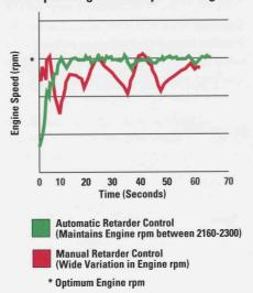
**Fuel Efficiency.** The engine provides additional retarding by running against compression on downhill hauls. During retarding applications the engine ECM does not inject fuel into the cylinders for exceptional fuel economy.
