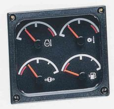
**Gauge Cluster.** Conveniently located gauge cluster maintains a constant display of vital machine functions, including:
