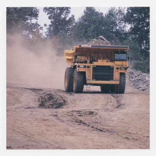
Integrated Braking System. The Cat oil-cooled braking system delivers reliable performance and control in the most extreme haul road conditions. The integrated system combines the service, secondary, parking brake and retarding functions in the same robust system for optimum braking efficiency.
