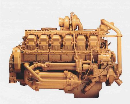
**Engine.** The Cat 3512B EUI twin turbocharged and aftercooled diesel engine delivers high power and reliability in the world's most demanding mining applications. The 3512B is a 16-cylinder, four-stroke design that uses long, effective power strokes for more complete fuel combustion and optimum efficiency.
