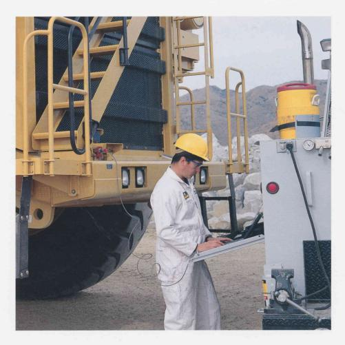
Servicing Ease. Easy access to daily service points simplifies servicing and reduces time spent on regular maintenance procedures. Enhanced serviceability and 500-hour service intervals are designed to increase machine availability and productivity.
