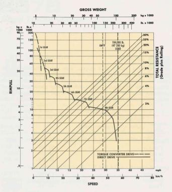
To determine gradeability performance: Read from gross weight down to the % of total resistance. (Total resistance equals actual % grade plus 1% for each 20 lb./ton (10 kg/t) of rolling resistance.) From this weight-resistance point, read horizontally to the curve with the highest obtainable speed range, then down to maximum speed. Usable rimpull depends upon traction available and weight on drive wheels.
