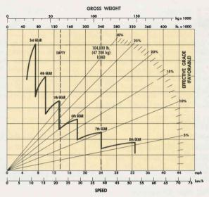
To determine retarder performance: Read from gross weight down to the % effective grade. (Effective grade equals actual % grade minus 1% for each 20 lb./ton (10 kg/t) of rolling resistance.) From this weight-effective grade point, read horizontally to the curve with the highest obtainable speed range, then down to the maximum speed. Retarding effect on these curves represents full application of retarder.
