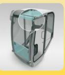
2 The top sliding part simply slides under the cab roof. There it is safely stowed.
