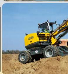
The Load Sensing hydraulics bring quality of performance into play: safe and sensitive excavation quickly becomes routine for the 95032.
