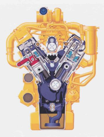
**3408E Tractor Engine.** The engine has the HEUI<sup>TM</sup> fuel system which uses hydraulically actuated electronically controlled unit injectors. The 3408E diesel engine has dual horsepower capability for the tractor, and provides the power and torque rise for excellent lugging in tough loading conditions.
