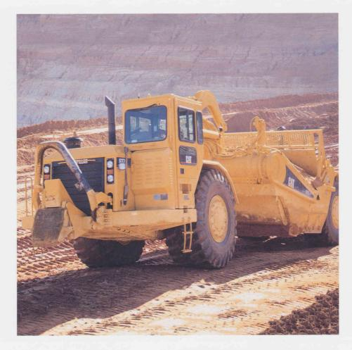
• The scraper transmission is electronically controlled by the tractor transmission and is synchronized to match the tractor transmission gear selection.
