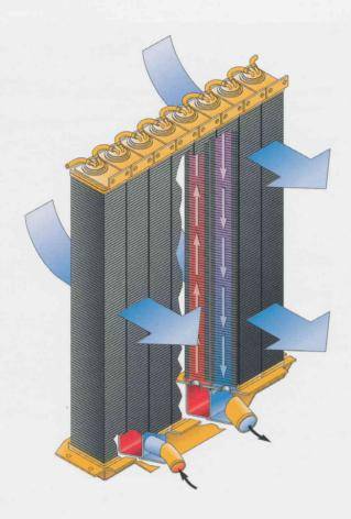
**Increased Performance.** Dual stage coolant flow process improves cooling capability by allowing coolant to pass on the air side of the radiator as well as the fan side. The coolant travels:
