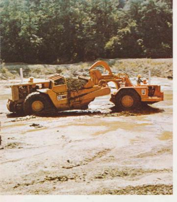
The heavy-duty scraper transmission is a planetary type featuring full torque converter drive with four ranges. Each range matches two of the tractor ranges. During turns when the scraper's tires have a shorter turning radius and must go slower than the tractor's, the converter drive automatically adjusts to the differential without lugging down or killing the rear engine. And the drive always assures high engine rpm, regardless of ground speed, to maintain a constant, high torque pushing power.
