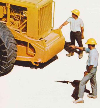
Another 627 performance feature is "automotive" follow-up type steering control with feel-of-the-road. This is compared with the "jerk steering" of Make "A".
