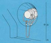
Fast fuel filler adapter—for high speed pressurized fueling.
