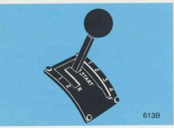
613B features four manually selected, power shift speed ranges forward and two reverse . . . and full torque converter drive for high torque and antistall performance.
