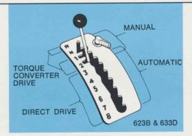
Cat 8-speed semiautomatic transmission combines automatic shifting with high torque multiplication and direct drive mechanical efficiency. Reverse, 1st and the highest desired gear are manually selected. The transmission automatically shifts up or down between 2nd and the highest selected gear. Reverse, 1st and 2nd gears are torque converter drive . . . providing powerful rimpull for loading and dumping. Gears 3 thru 8 are direct drive for quick acceleration and high hauling speeds.
