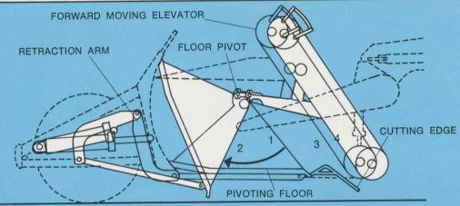
spreading or mass dumping. The scraper floor pivots (1-to-2) back and up from the fixed cutting edge. This action also serves to clean the bowl sides and back. At the same time, the elevator moves forward (3-to-4) and out of the way. This prevents material from being forced into the flights, and affords an even larger opening for mass dumping.
