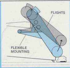
Cat's Flexible Mounting protects elevator flights and cutting edge against sudden shock. Elevator is free to swing upward to accommodate rocks or other large objects . . . quickly returns to position to keep loading the bowl.
