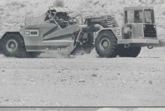
**The 613B** at 11 cu. yd. (8.4 m³) heaped, is mobile, versatile and economical to own and operate. The proven Cat 3208 engine and power shift transmission make it a reliable performer.
