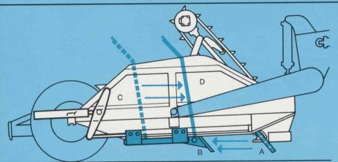
613B and 623B Eject in two smooth, fully - operator - controlled steps. (1) Scraper floor and cutting edge slide back (A-to-B) about half the floor's length for a large opening. (2) Simultaneously, the dozer-ejector moves (C-to-D) forward to the cutting edge, forcing out all materials, cleaning the sides and floor. Double-acting control cylinders give positive force in both directions. Fast and effective.
