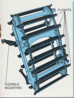
The 623B and 633D flights are modified box-section high-strength steel . . . the 613B has a rugged, modified triangular flight.
