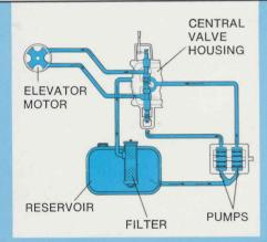
Hydraulic Drive System is sealed and filtered. Particles worn from pumps or motors are immediately caught by the filters. The circuit has no breather-type venting, no chance for dirt to enter the circuit to cause premature wear.
