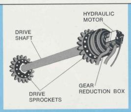
High-torque Hydraulic Drive turns the elevator at a relatively constant speed under heavy loads. This lets the operator select the best loading depth without continual adjustment. Leaves the cut smooth for easier, more efficient loading on the next pass.
