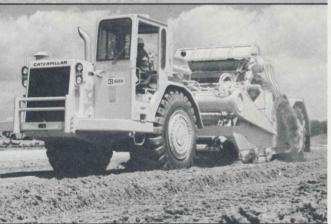
**The 623B** is a 22 cu. yd. (16.8 m³) heaped machine. The reliable 3406 engine, 8-speed semi-automatic transmission, variable capacity torque converter and cushion hitch arrangement keep it producing wherever you put it to work.
