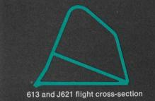
High-strength elevator has long life. The 613 and J621 flights are 100% high-strength steel in triangular construction for rigidity and resistance to wear. The 633C HT steel flights are modified box-sections with I-beam support running the full length of the faces—strongest in the industry. Rigid flight construction reduces bending and twisting which can hold chain out of line and shorten life of all components.
