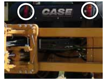
Rear road lights can be fitted on the stabilizer legs while traveling and on the cab when digging, providing maximum visibility and protection
