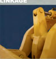
Z-Bar linkage transfers maximum force to the bucket to pry out har material. All loader linkage pins a to keep out abrasive dust and gri
