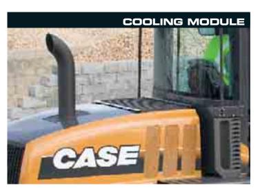
The Case E Series wheeled loaders benefit from a completely new design philosophy, with a mid-mounted cooling module situated behind the cab. Separate radiator cores for engine coolant, transmission oil, the aftercooler, air conditioning condenser and hydraulic oil cooler (optional) provide the most effective cooling solution, with a hydraulically-driven cooling fan pulling air through the individual cores.
