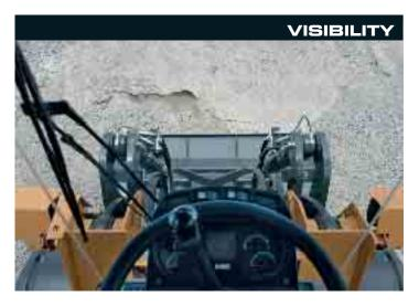
All Case E Series wheeled loaders benefit from a larger operator's cab, with up to 15% more floor area than the D series machines. The tapered design is longer and wider than previously, providing increased internal space for the driver. Reduced noise levels are among the quietest in the industry.
