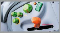
Accurate electronic hitch regulator (EHR) and electronic engine speed memory for recalling speeds during routine tasks.
