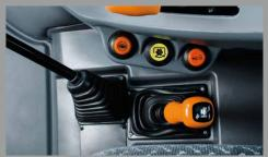
Electro-hydraulic activation of PTO, four-wheel drive and differential lock as standard (LS and GS).
