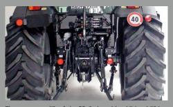
The rear power lift of the 5D Series with additional lifting cylinders lifts up to 3,600 kg and can therefore manage all common equipment in this power class.
