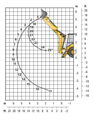
Lift Capacities are over-end values. Machine equipped with 4WD, OROPS, 1.34 m³ (1.75 yd³) general purpose loader bucket, 610 mm (24") heavy duty backhoe bucket and 1000 kg (2,200 lb) counterweight.
