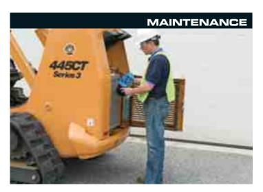
Regular service items can be easily accessed through a lift up panel on top of the engine cover and a full swing-out door to the rear of the machine. For more in-depth maintenance the entire cab structure can easily be tilted forward in less than a minute, to provide unparalleled access to the centre of the machine.
