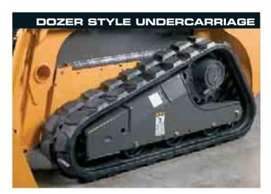
The rigid track frame with no moving parts reduces maintenance costs compared to suspension track systems.
