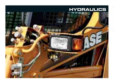
Gear pump and 3 spool open center system offer optimum hydraulic power. Standard auxiliary hydraulics (working at flow and pressure of the main system) drive most hydraulic attachments. For more hydraulic power demanding tools, optional high flow hydraulics can be specified for planers, stump grinders and other alike attachments. All CT's can share attachments with the popular Case skid steer range, XT's, 400 series and all other major brands, thanks to their universal coupler.
