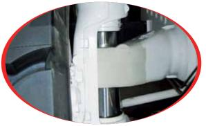
The engine brake, acting on the engine exhaust valves, turns the engine into a compressor and produces a modulated braking power according to the engine current push. It can develop a braking power of 380 HP at 2000 rpm. It is normally used to slow down the vehicle on flat terrains or downhill. It activates automatically when the accelerator pedal is released.
