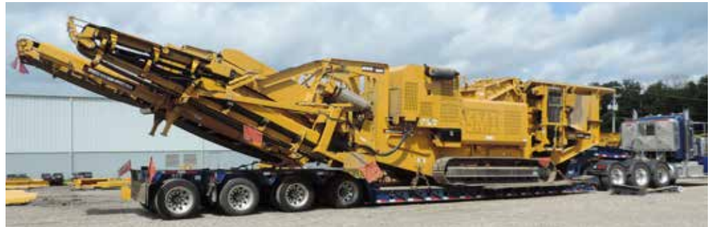
Recirculating conveyor swivels for transport.
