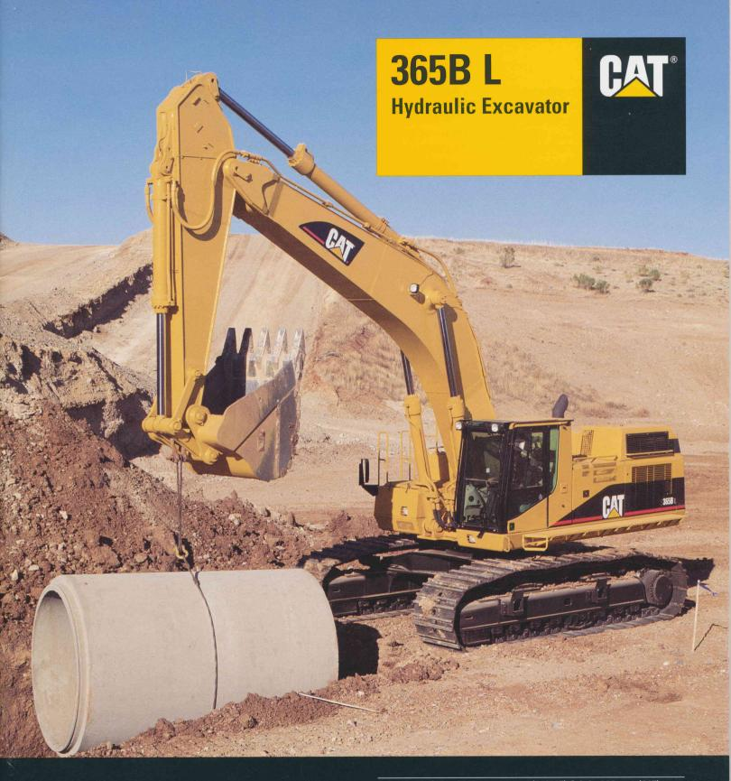
7.8 m (25'7") Reach Boom, 3.6 m (11'10") Stick, 900 mm (36") Track, and 1545 mm (60") 2.7 m<sup>3</sup> (3.6 yd<sup>3</sup>) GP Bucket Operating Weight 67 630 kg 149,000 lb Cat<sup>®</sup> 3196 ATAAC Diesel Engine
