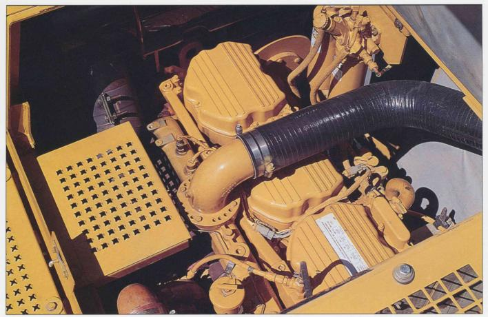
**Innovative Cat 3196 ATAAC diesel engine** delivers large-engine performance from a compact engine design. The six-cylinder 287 kW (385 hp) engine is turbocharged and air-to-air aftercooled. With high horsepower and low displacement, this engine provides excellent fuel economy and durability that can significantly reduce operating costs.
