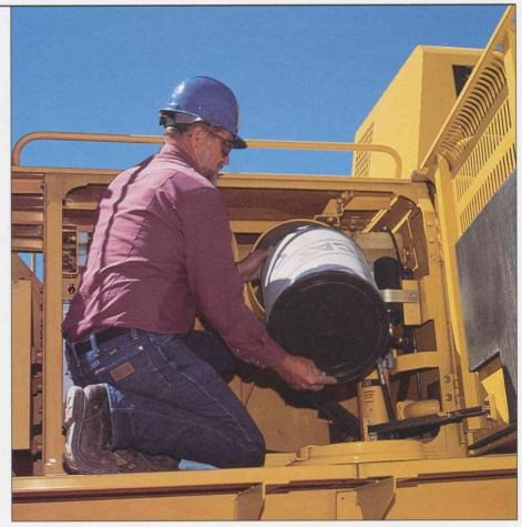
Water separator removes water from fuel even when under pressure and is located in the battery compartment for easy access.
