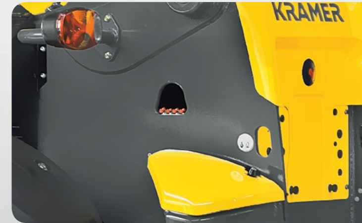
Joint lubrication points: Oscillating axle, lifting and balance cylinder can be lubricated in one operation. It is not necessary to lift the telescopic arm.
