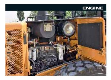
The 1221E is powered by a Tier III compliant 11 litre Cummins engine, delivering a maximum output of 320 net hp (239kW). Electronic control with high fuel injection pressures ensure cleaner, more efficient burning, resulting in maximum output with greatly reduced exhaust emissions and fuel consumption. The machine is compatible with the Case electronic service tool (EST) for rapid diagnostics and minimum downtime.
