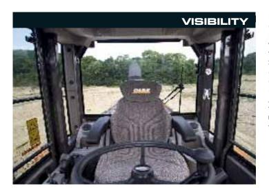
Pillarless top to bottom glazing to the front and both sides of the cab offers an excellent view of the bucket corners or attachment. Powerful windscreen wipers keep the main window clear in all weathers and the fenders prevent muck from the wheels being thrown onto the windows.
