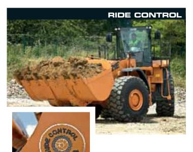
As a leader in ergonomic design, all Case wheel loaders can be specified with Ride Control, a system that allows the lift arms to float while the machine is moving. Ride Control reduces shock loadings in the machine, and the bounce that is felt in the cab, reducing fatigue for the operator and prolonging component life. Ride Control allows the operator to drive at higher speeds during load and carry operations, improving load retention of material and boosting productivity.
