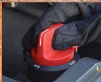
Battery cut-off switch
