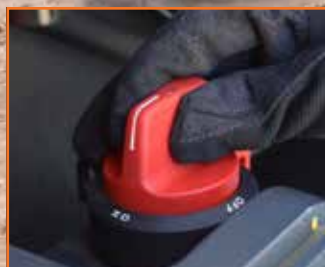
Battery cut-off switch
