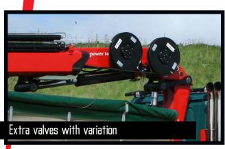
A well-known and usual hose routing to the end of the extensions means that 1 or 2 extra valves are fed in sturdy hose guides alongside the jib extension system. If further efficient protection of the hoses is required, 1 or 2 extra valves can be fed in internal hose reels and lie particularly well protected. In case of more than 6 hydraulic extensions or a reach of approx. 17 m, 1 or 2 extra valves will be fed in external, smooth-running and efficient hose reels.
