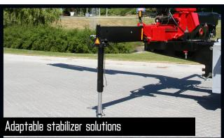
The stabilizer legs of the crane are to ensure stability - however they still have to be sturdy, easy to handle and must not take up too much space when not in use. Therefore you can choose between fixed stabilizer legs, manual swing-up stabilizer legs to 30/60° or manual swing-up stabilizer legs to 180° with gas spring. Stabilizer beams can be freely selected as hydraulically extensible or manually extensible, also in connection with the sophisticated EVS stability monitoring.
